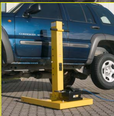
Lifting on the Sill
